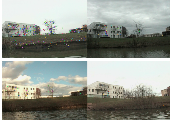
Figure 11: Snapshots of a scene along the lakeshore. The colored dots are the only features that could be matched. top left) The result of feature matching for two nearby images in the same survey. top right and bottom) The result of feature matching between this image and the top left image.
