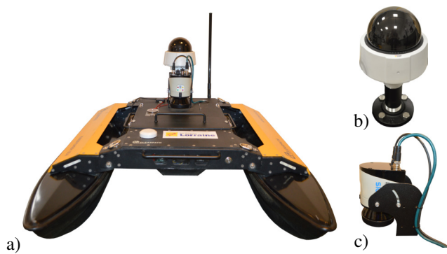
Figure 2. a) Front view of our Clearpath Kingfisher and side views of b) the PTZ camera, and c) the 2D LiDAR. A survey is initiated using a computer connected via the wifi antennae in the back. As the motor in each pontoon propels the robot, the camera pans starboard (or port for the island). The laser range-finder measures the ranges to obstacles, which are used to maintain a 10m distance to the shore. The GPS, the compass, and the IMU measure trajectory values while the computer inside the waterproof compartment records all of it.
