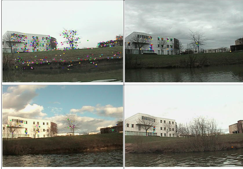
Fig. 3. Snapshots of a scene along the lakeshore. The colored dots are the only features that could be matched. top left The result of feature matching for two nearby images in the same survey. top right and bottom The result of feature matching between this image and the top left image.
