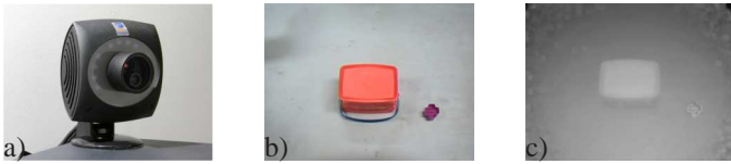
Fig. 3. The robot's vision system: a) the 3D camera (a ZCam [44]); b) a color image of the red non-container captured by the camera when mounted on the robot; c) the depth image corresponding to b).
