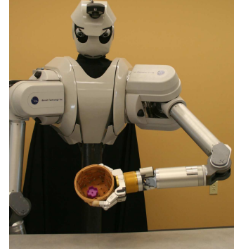
Fig. 1. The upper-torso humanoid robot, shown here shaking one of the objects used in the experiments. The small plastic block inside the object produces auditory and visual events, which the robot can detect and use to categorize the object as a container.
